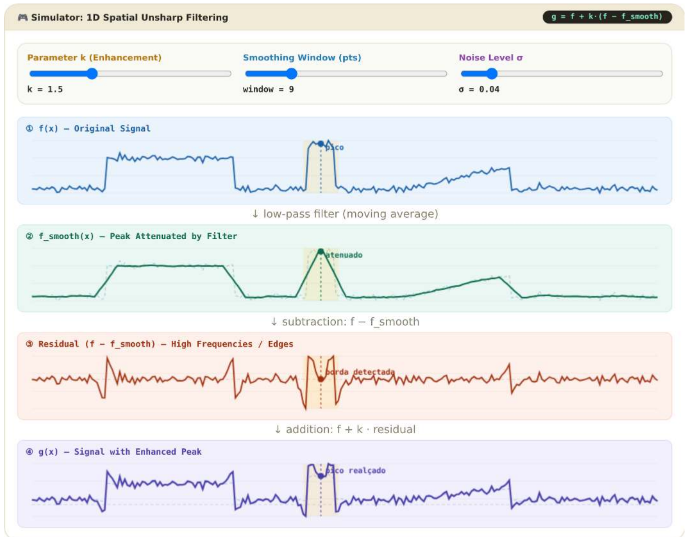
Figure 3.15: Simulator: 1D Spatial Enhancement Filtering (Unsharp Masking and High-Boost)
